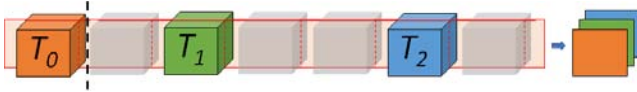
Fig. 4: 3TP Slice creation: slices extracted from the pre-contrast ( t_0 ), from 2 ( t_1 ) and 6 minutes ( t_2 ) after the CA injection volumes are fused in a 3 channels image.
